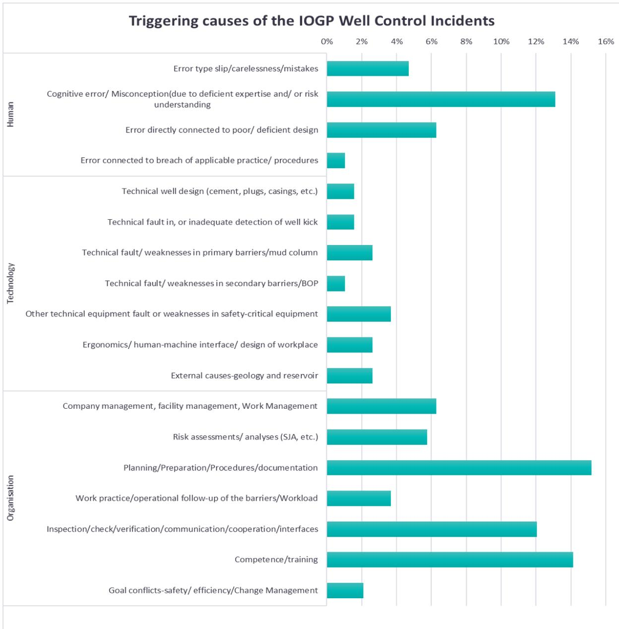
**Figure 5 - Well Control Incidents – Failure Points<sup>5</sup>**
