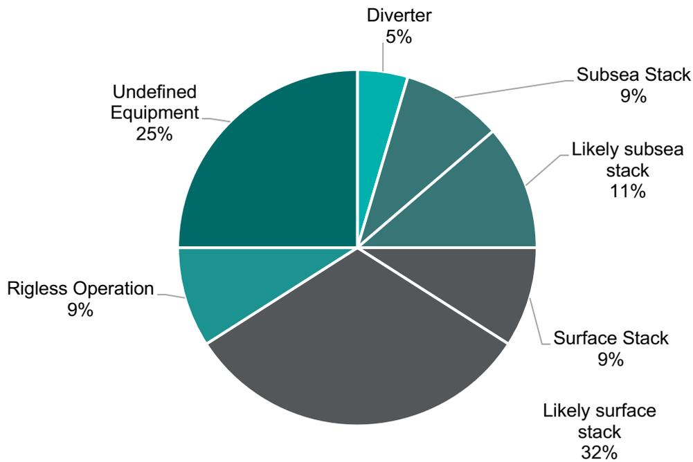
**Figure 4** - Well Control Incidents vs. Well Control Equipment Used
