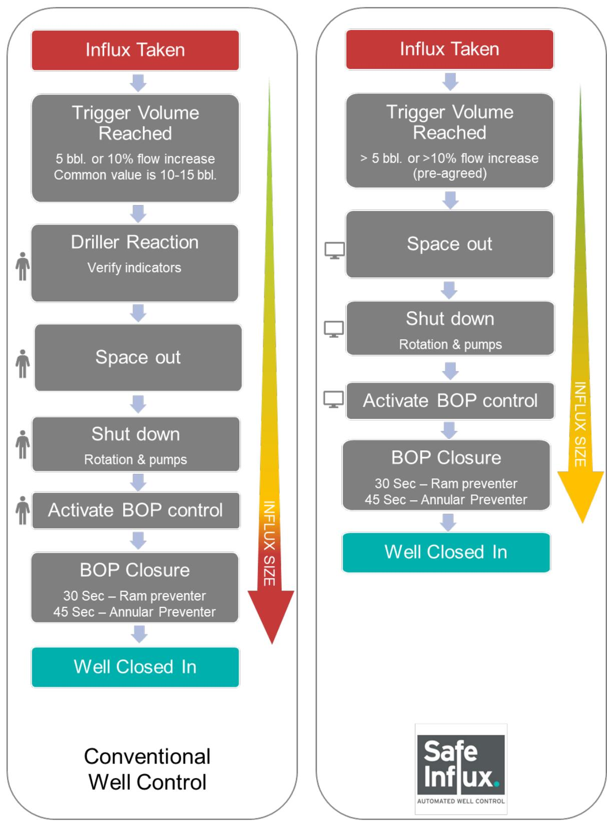
Figure 9 - The effect of Automation on Influx Size
